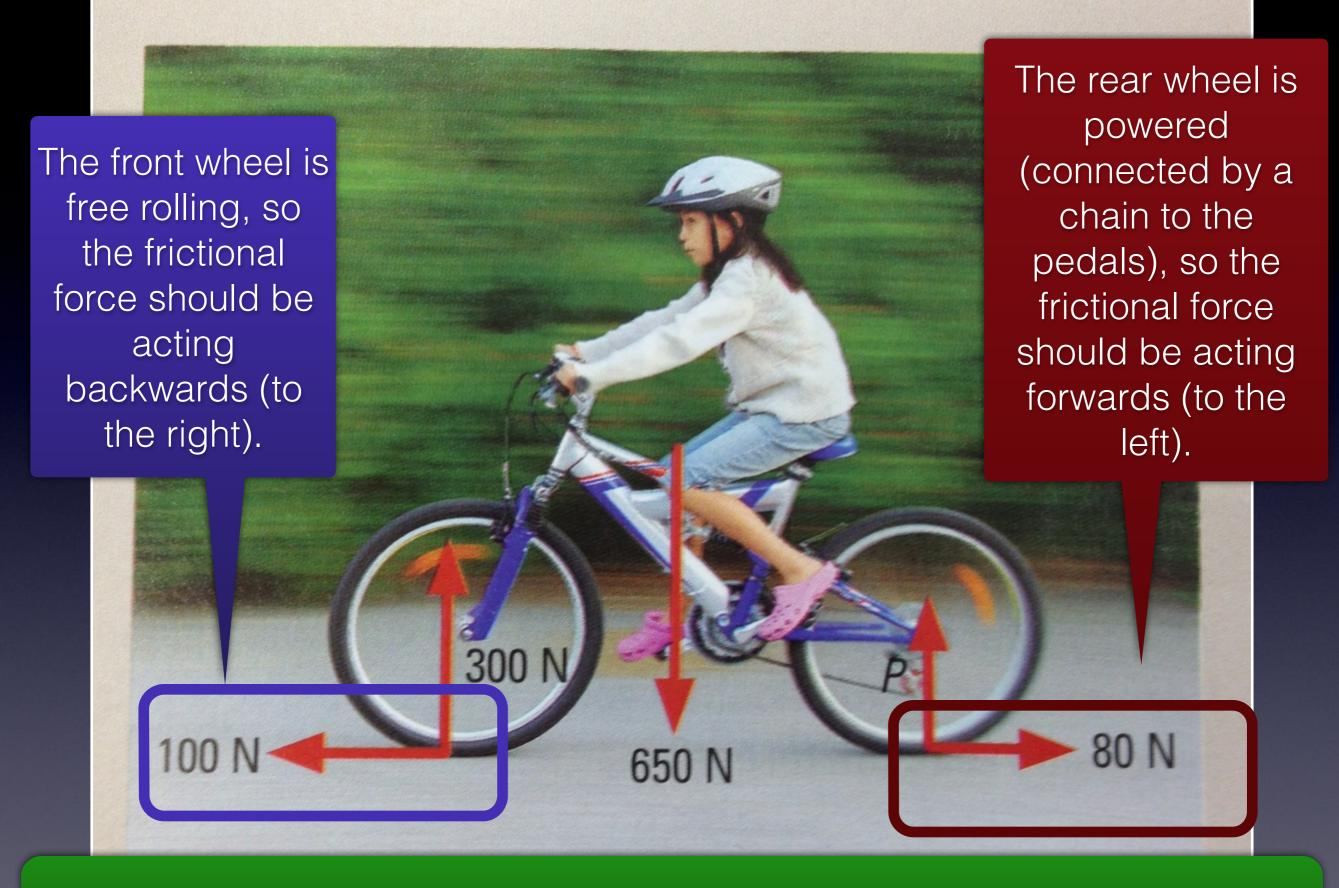
If the bicycle is accelerating (moving faster), the forward frictional force) must be greater than the backward frictional force (plus air resistance)
